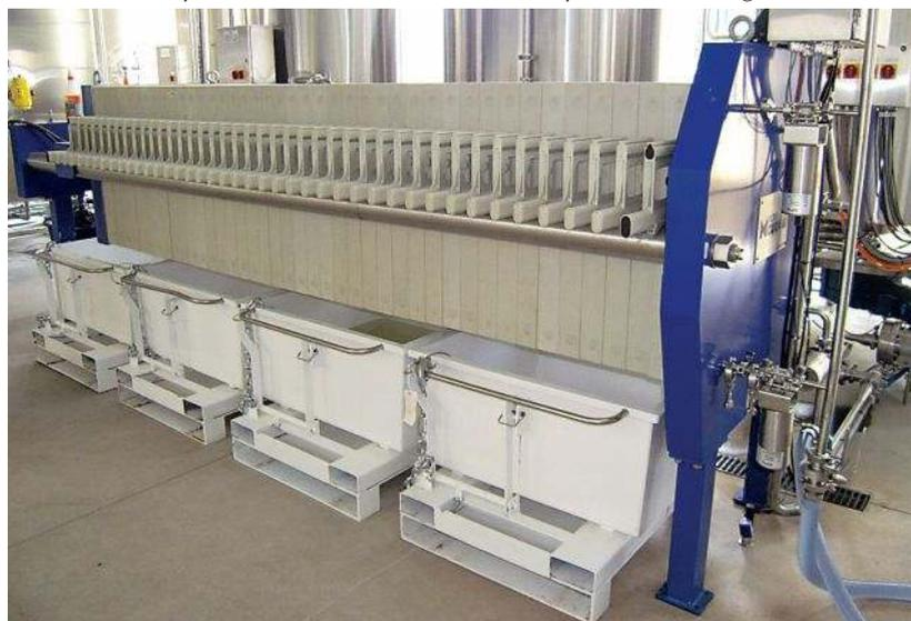
The brewing system is four vessels with mash tun, mash filter, boil kettle and whirlpool, all running via Siemens BRAUMAT Compact process control system. What is most exciting about this brewing system is the Meura mash filter that replaces a traditional lauter tun as employed by 99 plus percent of the brewing systems in the USA. No other brewery in Michigan has one, and there are very few in America (yet 25% of
